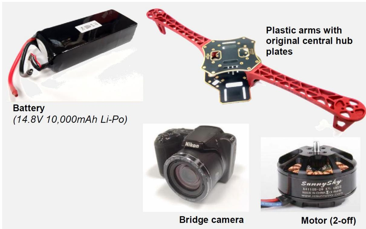
Figure 2: 4 kg class drone components
