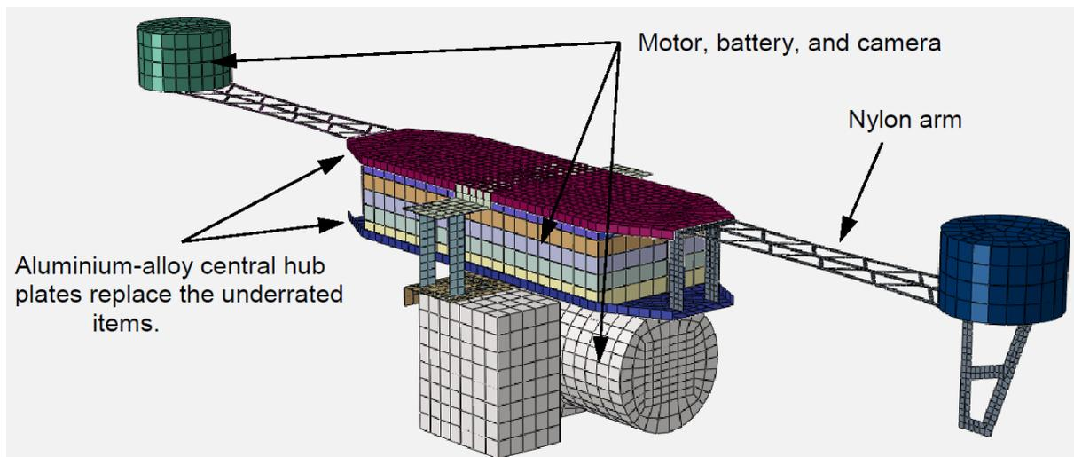
Figure 3: 4 kg class drone components model
